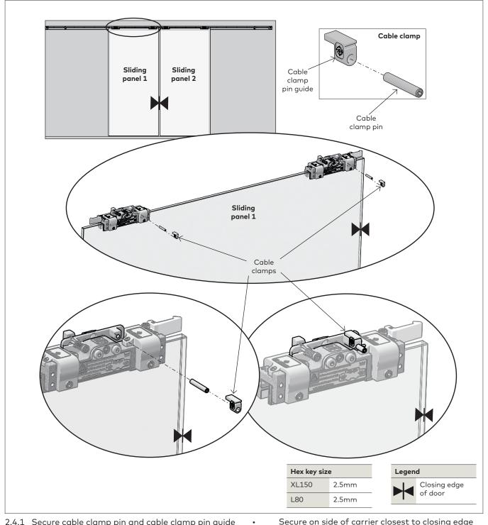
2.4.1 Secure cable clamp pin and cable clamp pin guide into carrier as shown.
