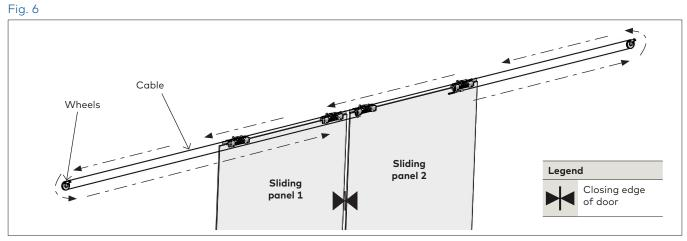
2.6.1 Thread cable around wheels in direction as shown.
